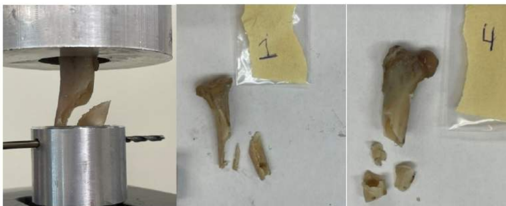
Fig. 7. Tensile Tests Results (a) Close View of the Oblique Fracture on Batch 1, Sample 1 (b) Oblique Fracture on Batch 3, Sample 1 (c) Oblique Fracture on Batch 3, Sample 4
