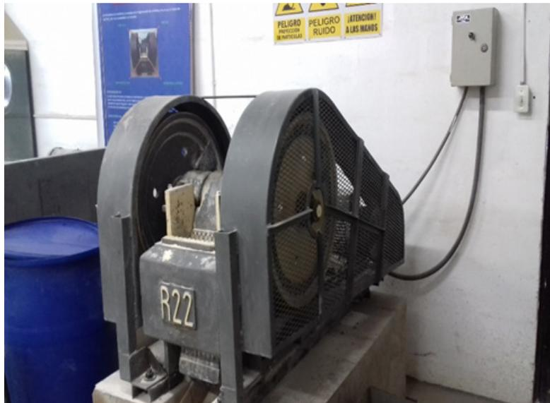
**Fig. 2. MEM R 22 Jaw Crusher**
