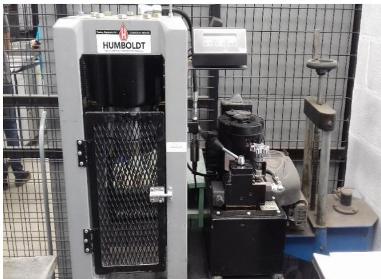
**Fig. 4. Humboldt Compressive Strength Testing Equipment**
