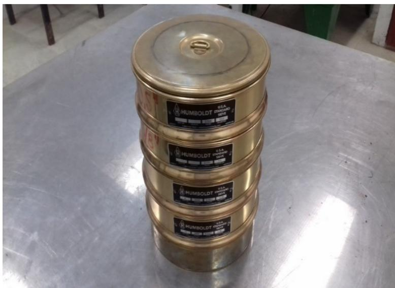
**Fig. 3. Set of sieves for granulometric classification**
