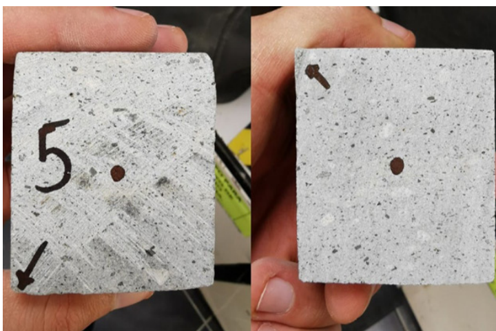
Fig. 3. Rock specimen after cutting
