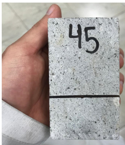
Fig. 2. Rock specimen ready for cutting
