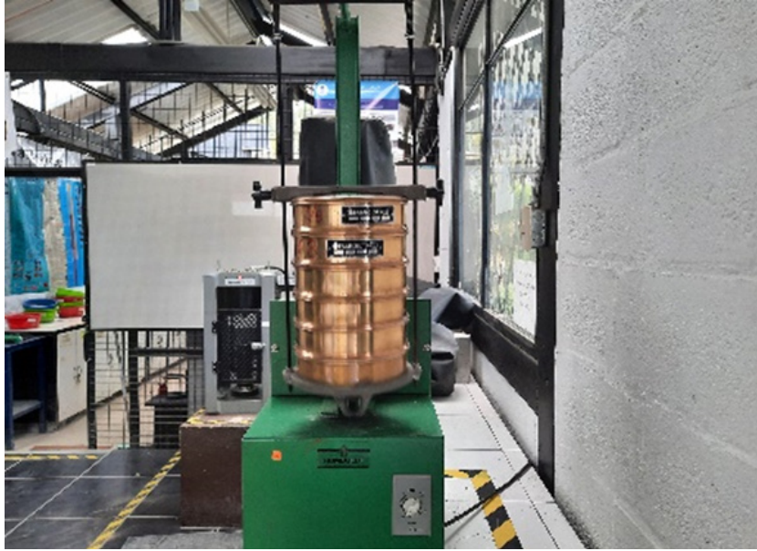
Fig. 4. Classification process by electric sieve
