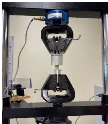
Fig. 2. Tensile Test Calibration and Setup
