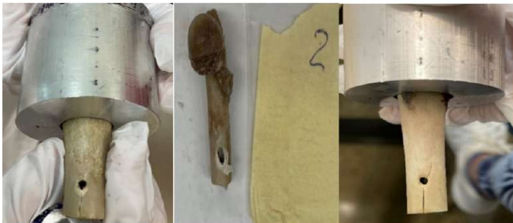
Fig. 6 (a) Longitudinal Fracture on Batch 3, Sample 1 (b) Longitudinal Fracture on Batch 3, Sample 2 (c) Longitudinal Fracture on Batch 3, Sample 3
